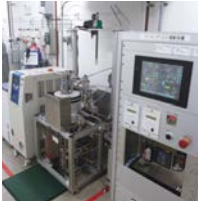
Equipment for testing friction and wear in a hydrogen atmosphere
