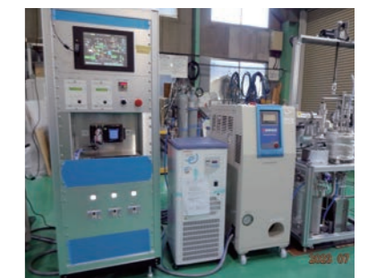
Friction and wear test equipment in a hydrogen atmosphere
